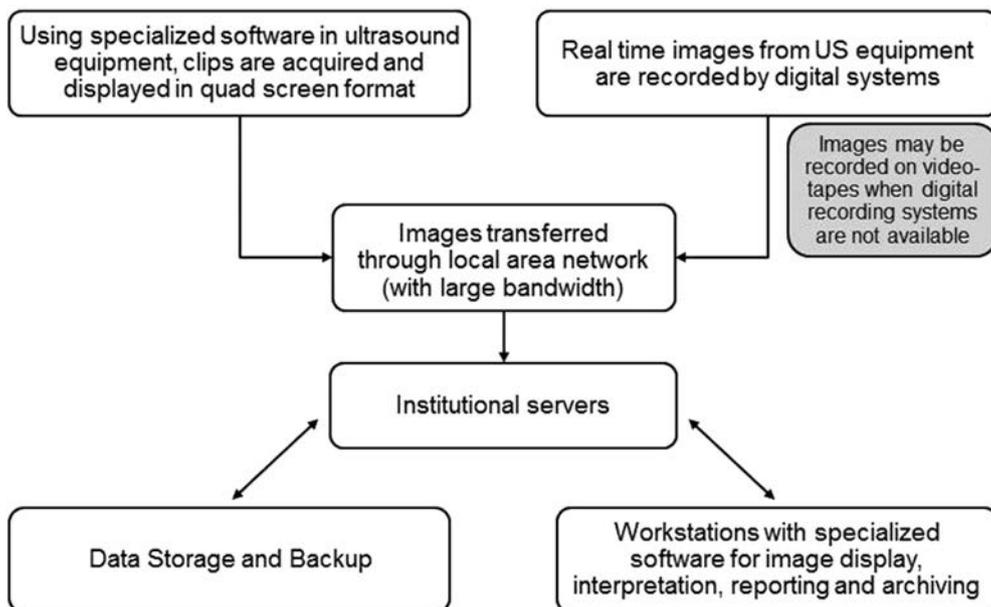
**Figure 3** Systems architecture from a stress echocardiography laboratory. The digital images may be transferred from the ultrasound system through a computer network to departmental servers, then to computer workstations for their offline analysis and interpretation. Network systems with large bandwidth and servers with large archiving capacity are required. Serial stress examinations may be digitally archived and retrieved for side-by-side comparison of images.
